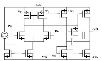
Fig. 5: pipeline amplifier schematics.
