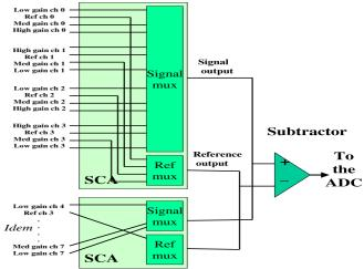
Fig. 2 : output cabling for 8 SCA channels
