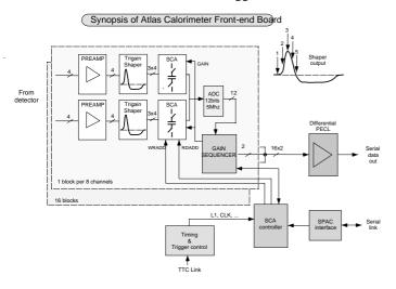
Fig. 1: block diagram of the Front-end board
