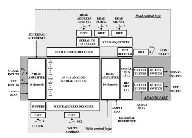
Fig. 3: analog memory architecture.
