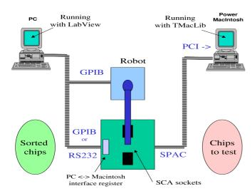
Fig. 7: production test bench setup
