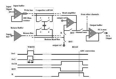
Fig. 4: channel block diagram
