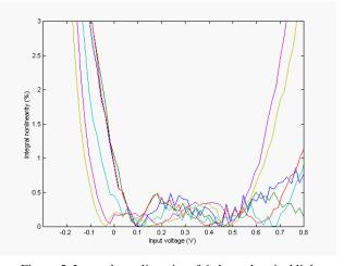
Figure 5: Integral non-linearity of 6 channel optical link
