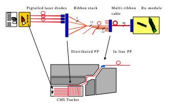
Figure 2: Optical link architecture.
