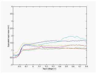
Figure 4: Equivalent input noise characteristic of 6 channel link
