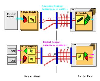
Figure 1: CMS-Tracker read-out and control system
